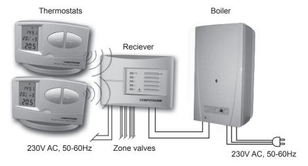
The device can be programmed according to customer-specific requirements so that the heating/cooling system heats/cools your residence or office to the required temperature at the dates and times specified by you, to reduce energy costs while maintaining comfort. Separate temperature programs can be prepared for each day of the week. For each day, beside 1 fixed switching time, 6 adjustable switching times can be set and a different temperature can be assigned to all 7 switching times.
