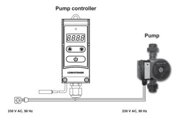
**Warning!** Always take into account the loadability of the controller relay when connecting (10 A (3 Inductive load)) and follow the instructions of the manufacturer of the pump which you would like to control.
