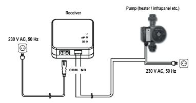
**ATTENTION!** Always consider the loadability of the receiver unit and follow the manufacturer's instructions of the heating or cooling equipment. The device must be installed and connected by a qualified professional!
