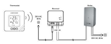
The effective range of the transmitter incorporated in the thermostat is approximately 100 m in open terrain. This distance may become considerably shorter within a building, especially when a metal structure, reinforced concrete or adobe wall stands in the way of radio waves.
