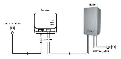
If you would like to operate an old boiler or any other device that has no connection points for thermostats, then the **NO** and **COM** connection points of the thermostat should be connected to the mains cable of the device, similarly as a switch would be connected.
