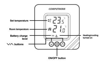
The device consists of two units. One of them is the portable control unit (thermostat), while the other unit is the receiver that controls the boiler. Because there is a wireless (radio-frequency) connection between the two units, no cable is required between the thermostat and the boiler. The two units have been tuned in the factory. The trouble-free operation is ensured by its own security code. The installation and connection of the receiver unit is described in **Chapter 8**.
