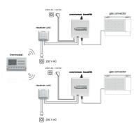
When you are able to establish wired connection between the gas convectors, you can also set up the system by using fewer **COMPUTHERM Q7RF (RX)** receiving units as shown in the figure below.
