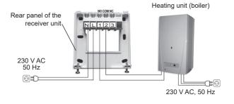
If you would like to operate an old boiler or any other device that has no connection points for thermostats, then the 1 (NO) and 2 (COM) connection points of the thermostat should be connected to the mains cable of the device, similarly as a switch would be connected, as shown in the figure below.
