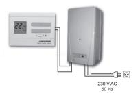
simple, conventional thermostats. In heating mode, in accordance with the selected switching sensitivity, the thermostat switches the boiler or any other appliances on and off below and above the adjusted temperature, respectively, and contributes to reduce energy costs while maintaining comfort. In cooling mode it switches the opposite way.
