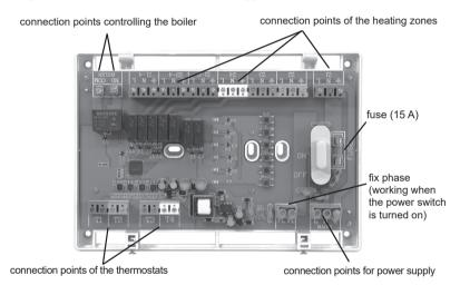
In case of using electro-thermal zone valves that operate slowly and all the zones are closed when the boiler is inactive, then the boiler should be started with a delay in order to protect the pump of the boiler. In case of using electro-thermal zone valves that operate fast and all the zones are closed when the boiler is inactive, then the valves should close with a delay in order to protect the pump of the boiler. See Section 5 for more information on the delay funcions.
